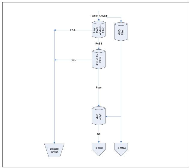
Figure 7-1. I210 Receive Filtering Flow Chart
