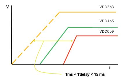
Figure 12-24.Internal SVR Power-Up Sequence
