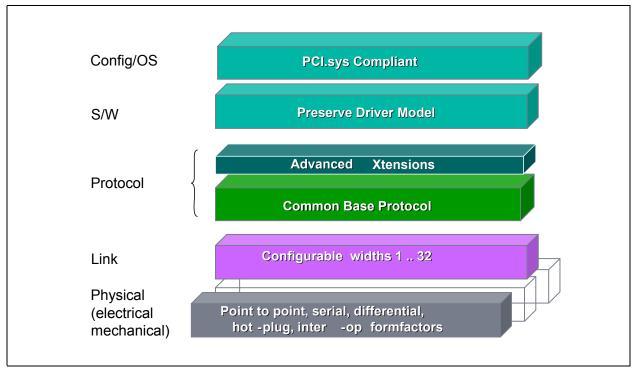
Figure 3-1. PCIe Stack Structure
