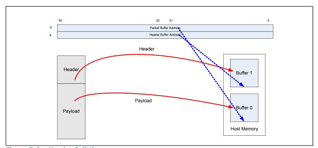
Figure 7-8. Header Splitting
