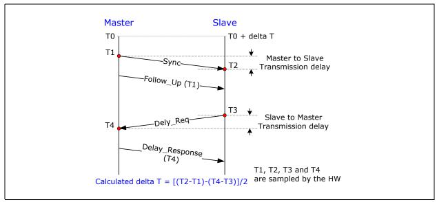
Figure 7-20. Sync Flow and Offset Calculation
