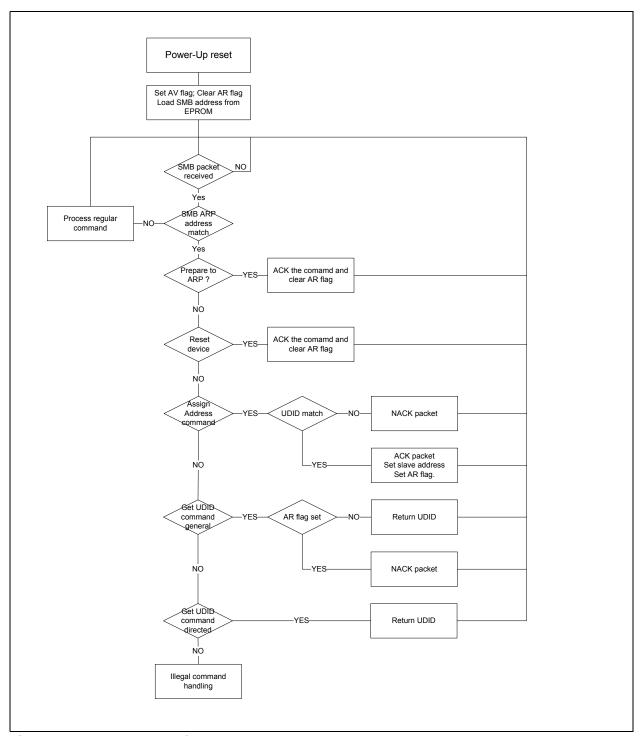
Figure 10-3. SMBus ARP Flow
