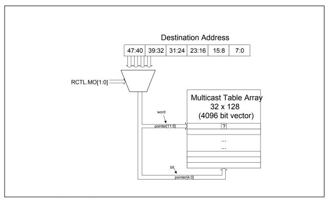
Figure 8-1. Multicast Table Array
