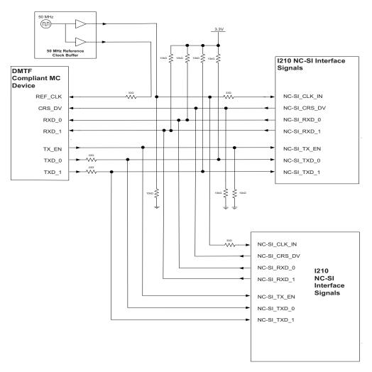
Figure 12-17.NC-SI Connection Requirements - Multi-Drop Configuration
