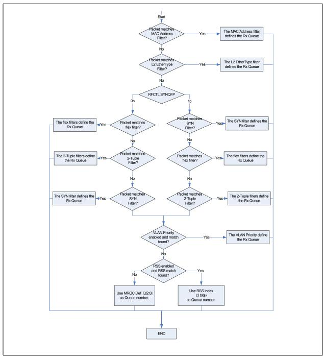
Figure 7-5. Receive Queuing Flow
