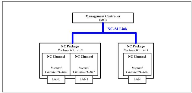
Figure 10-5. Two NC Packages (Left, with Two NC Channels and Right, with One NC Channel)
