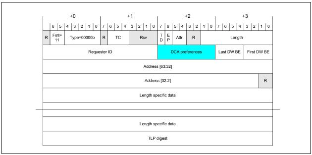
Figure 7-19. PCIe Message Format for DCA
