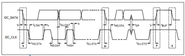
Figure 11-3. I<sup>2</sup>C I/F Timing Diagram
