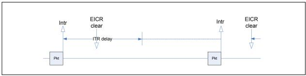
Figure 7-17. Light load, Interrupts Immediately on Packet Receive
