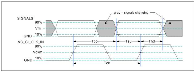
Figure 11-5. NC-SI Timing Diagram
