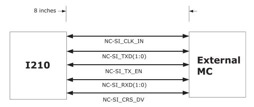
Figure 12-19.NC-SI Trace Length Requirement for Direct Connect
