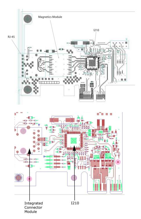
**Figure 12-14.Layout for Discrete Magnetics**
