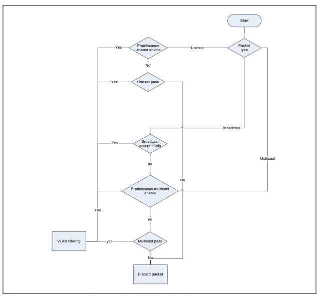
Figure 7-2. Host MAC Address Receive Filtering Flow Chart
