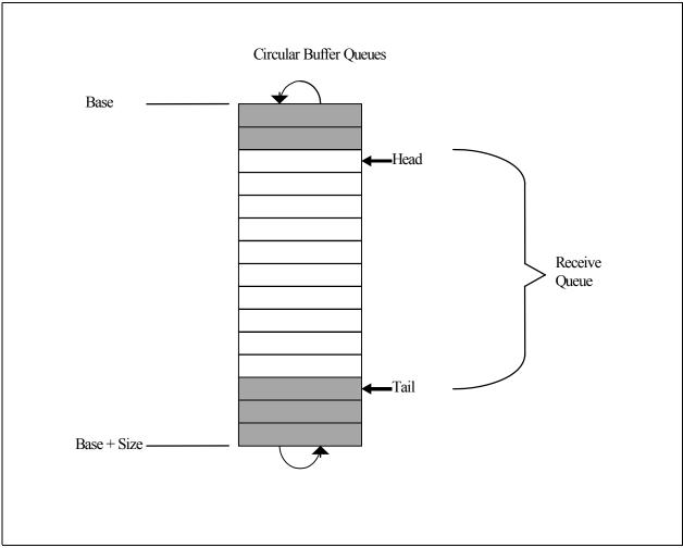
Figure 7-7. Receive Descriptor Ring Structure
