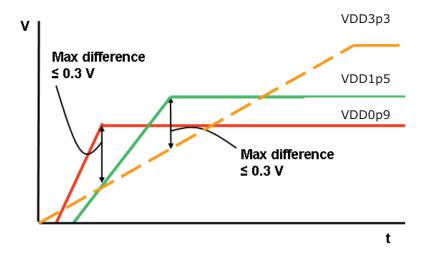
Figure 12-23. External Voltage Regulator Power-up Sequence
