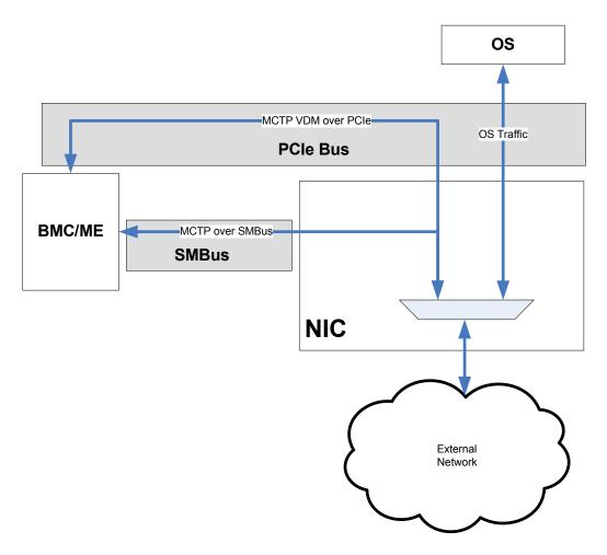
Figure 10-8. MCTP Connections of the I210
