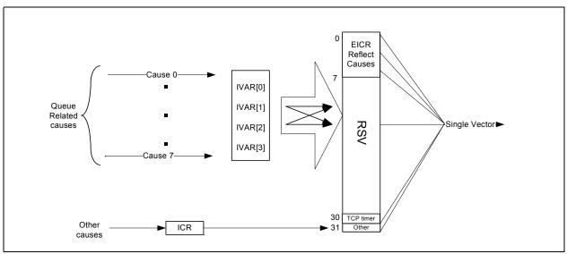
Figure 7-13. Cause Mapping in Legacy Mode
