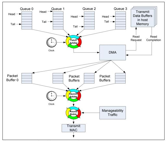
Figure 7-11. Transmit Architecture Qav Mode
