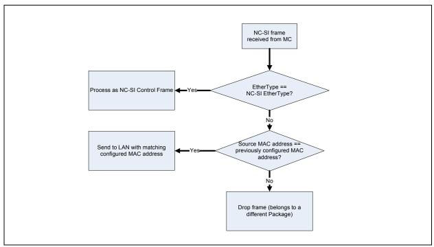
Figure 10-6. NC-SI Frames Receive Flow for the NC
