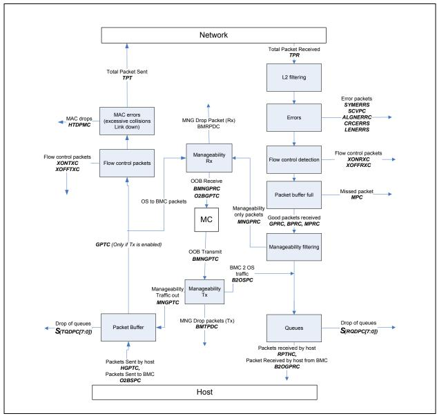
Figure 7-24. Flow Statistics Flow Statistics
