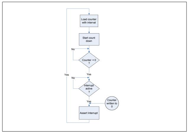
Figure 7-15. Interrupt Throttle Flow Diagram
