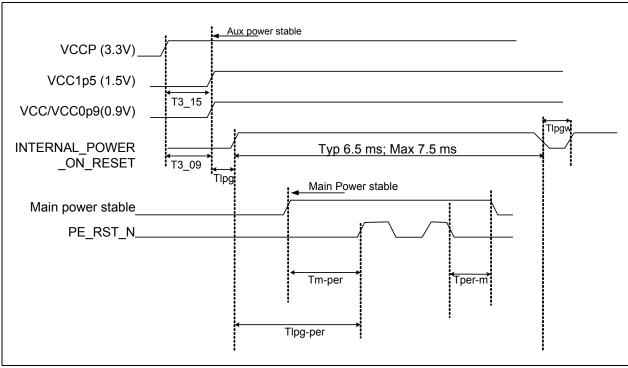
Figure 11-1. Power and Reset Sequencing
