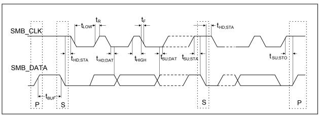
Figure 11-2. SMBus I/F Timing Diagram
