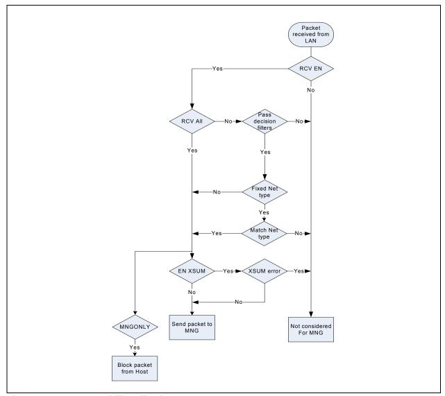
Figure 7-4. Manageability Filtering
