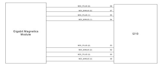
Figure 12-11.I210 Gigabit Magnetics Module Connections
