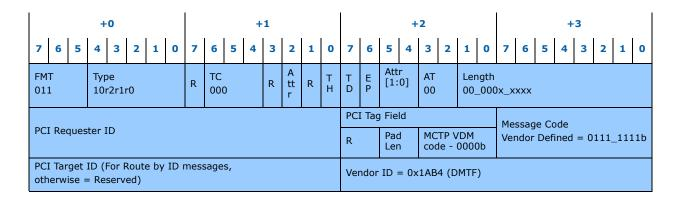
Figure 3-2. MCTP over PCIe VDM Header Format
