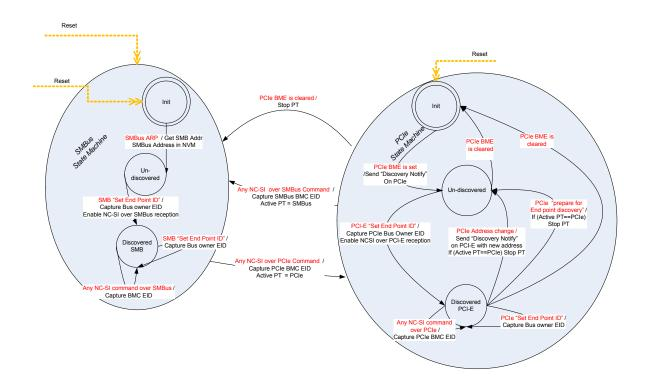
Figure 10-10.MCTP Bus Transition State Machine
