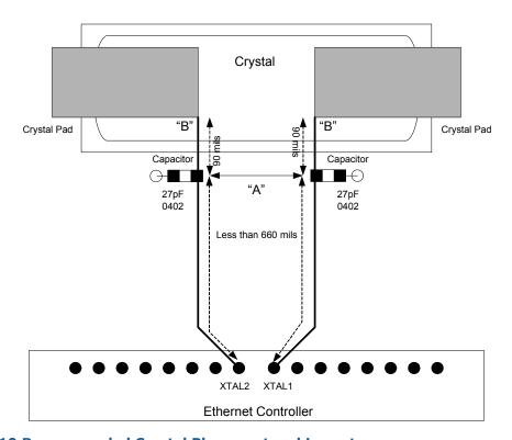
Figure 12-10.Recommended Crystal Placement and Layout
