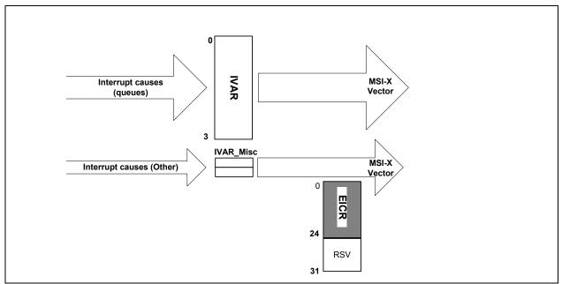
Figure 7-14. Cause Mapping in MSI-X Mode
