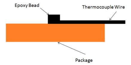
Figure 13-26.Technique for Measuring T<sub>case</sub> with 0° Angle Attachment, No Heat Sink
