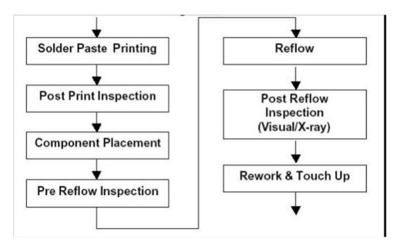
Figure 12-25. Assembly Flow
