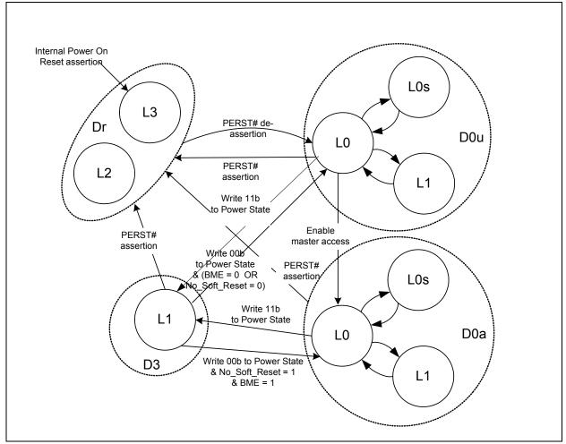
Figure 5-2. Link Power Management State Diagram
