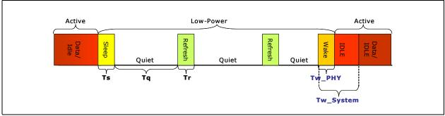
Figure 3-14. Energy Efficient Ethernet Operation
