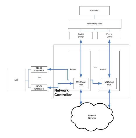
Figure 10-2. OS-to-MC Diagram
