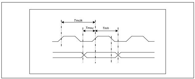
Figure 11-7. MDIO Input AC Timing Diagram
