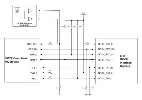
Figure 12-16.NC-SI Connection Requirements - Single-Drop Configuration
