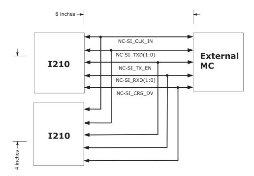
Figure 12-20.NC-SI Trace Length Requirement for Multi-Drop
