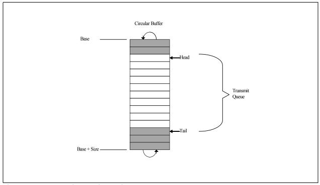
Figure 7-10. Transmit Descriptor Ring Structure
