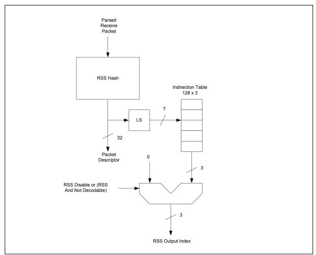
Figure 7-6. RSS Block Diagram
