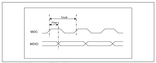
Figure 11-8. MDIO Output AC Timing Diagram
