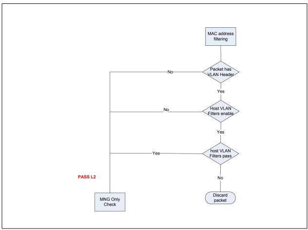
Figure 7-3. I210 VLAN Filtering
