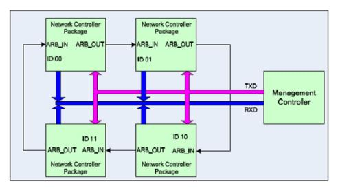
Figure 12-18.NC-SI Connection Requirements - Hardware Arbitration
