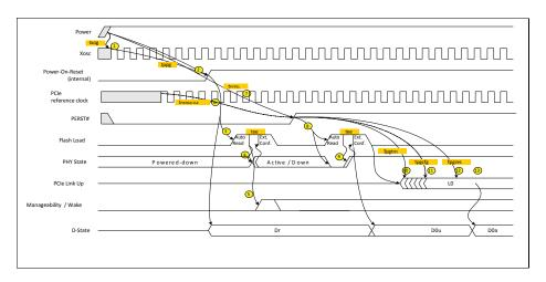
Figure 4-2. Power-Up Timing Diagram
